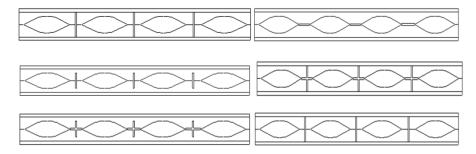
With reference of paper, Titled Optimization Of Opening Size For Castellated Beam With Sinusoidal Openings by P. D. Kumbharand A. M. Jamadar (Reference 10), the optimum parameters of Castellated Beam with Sinusoidal openings are selected for the analysis are as follows:
